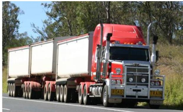
Image: Typical Triple Road Train Configuration
